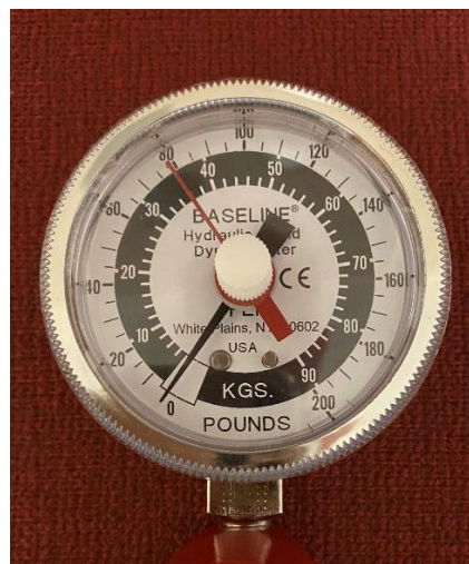
Figure 2: An example of a gauge reading when the dynamometer is used to measure grip strength. The black hand of the dynamometer shows the force applied during testing, and the red hand remains in the position corresponding to the maximum force exerted. When no force is applied, as in the image shown, the black hand gives the offset from zero that must be subtracted (approximately 79 lbs for the maximum and 3 lbs for the offset in the image shown).
