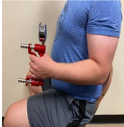
Figure 1: Demonstration of the standard AMA Guides method for determining grip strength using a hand dynamometer.
